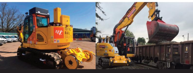
The GOS DX140 and DX235 Series conversions are UK Road/Rail conversions of Doosan standard tracked hydraulic excavators.
