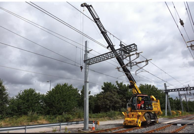
Renowned for its innovative road/rail vehicles (RRV's) over many years, GOS uses the well-proven Doosan DX170W-7 wheeled excavator as the base for a multi-purpose hydrostatic drive machine to match all challenging work applications.
